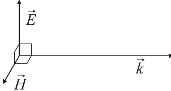
**Fig. 2.2** Relative orientations of the electric and magnetic fields and the wavevector. Reproduced, with permission, from Barnett(2009).
